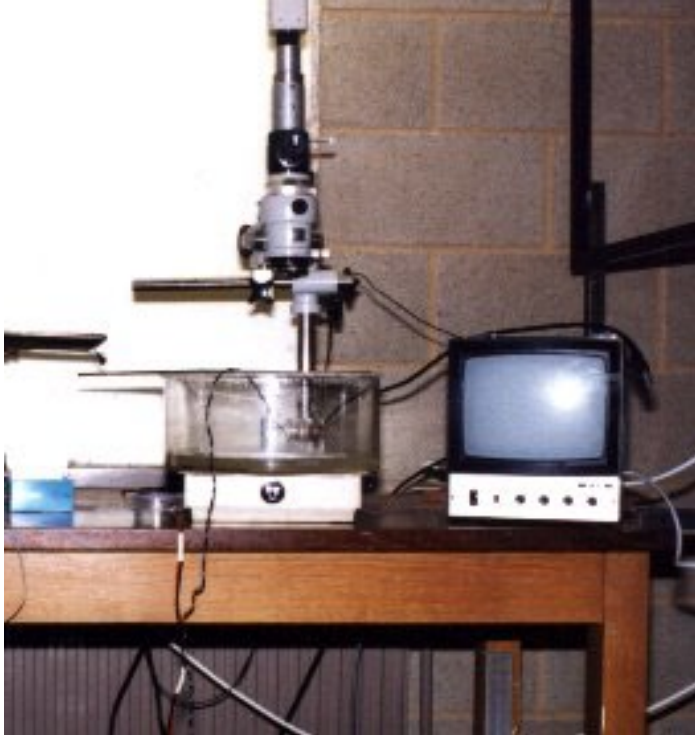
Fig 2.5 Photograph of oviposition humidity tank assembly with Tessonvar microscope, video camera and monitor
